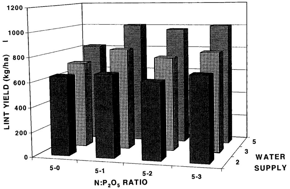
Figure 6. Cotton lint yield response to nitrogen-phosphorus ratios as a function of irrigation water supply.
