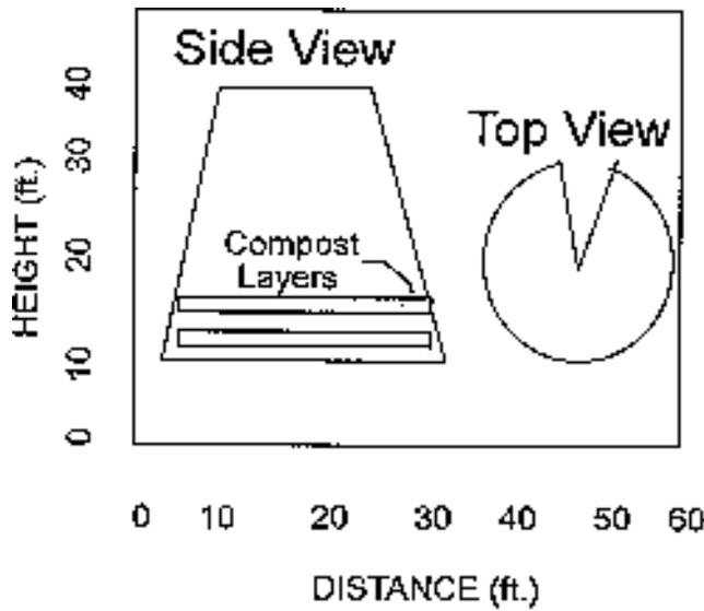
Fig. 1. Schematic diagram of a Lipsey® compost pile.
